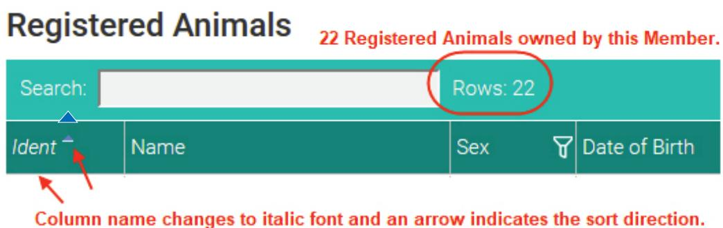
The screenshot shows a table header with four columns: 'Ident', 'Name', 'Sex', and 'Date of Birth'. The 'Ident' column has a blue arrow pointing down and left, indicating it is sorted in descending order. The 'Rows: 22' text is circled in red. The table body contains a search bar and a row of summary statistics.
